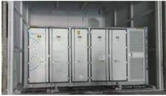
Figure 26 Battery compartment IP5X dust test
